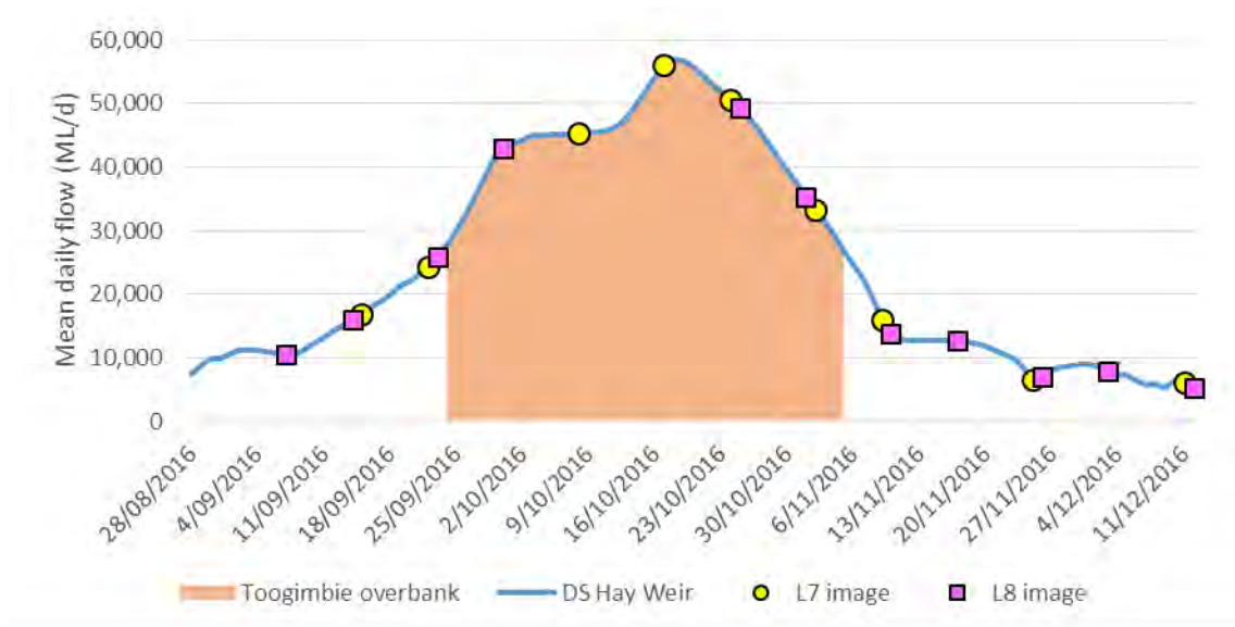
Figure 41. Hydrograph of 2016 flood event, recorded at DS Hay Weir, indicating period when flow exceeded commence to flow threshold at Toogimbie.
